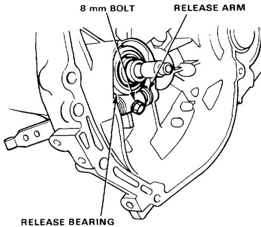
3. Separate the release arm from the bearing by removing the clip from the holes in the release bearing.
