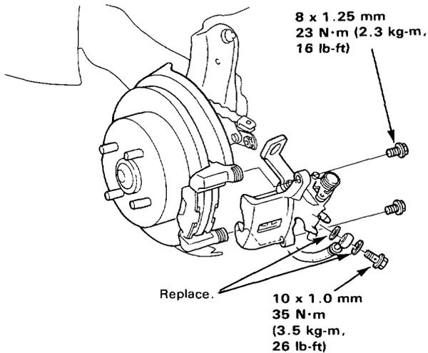
5. Remove the pad spring from the caliper.
