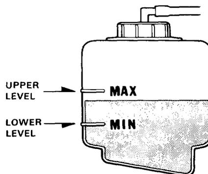
2. Supply the coolant reservoir tank with coolant to "MAX", if the coolant level is lower than "MIN" or near to "MIX".
