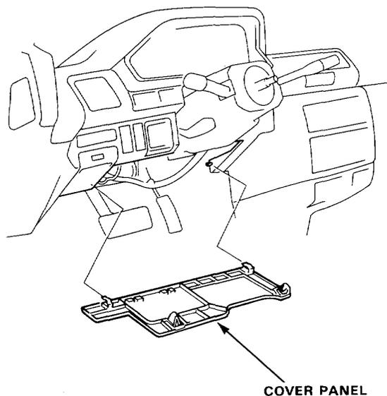
5. Remove the steering joint cover.
