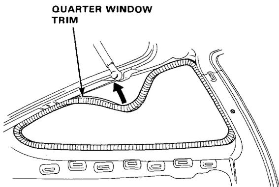
8. With a sponge, apply a light coat of body primer to the original adhesive remaining around the window opening flange.
