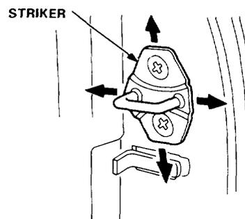
**NOTE:** Hold the outside handle out and push the door against the body to be sure the striker allows a flush fit.
