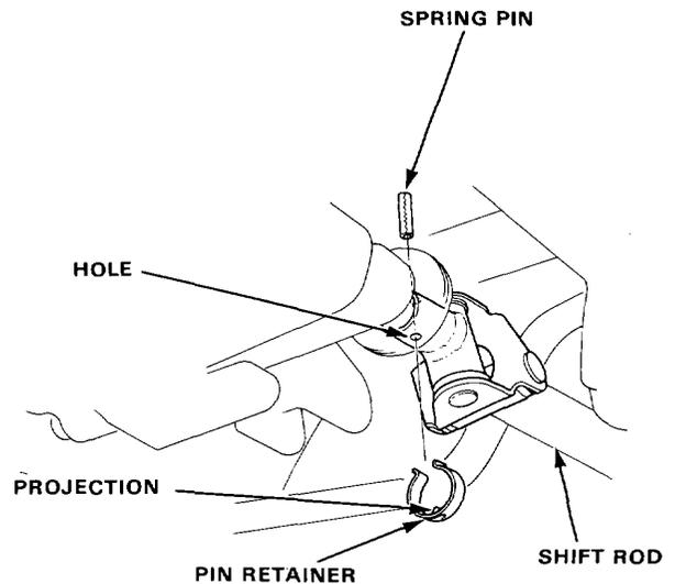
NOTE: On reassembly, reinstall the pin retainer after driving in pin and be sure that the projection on the pin retainer is in the hole.
