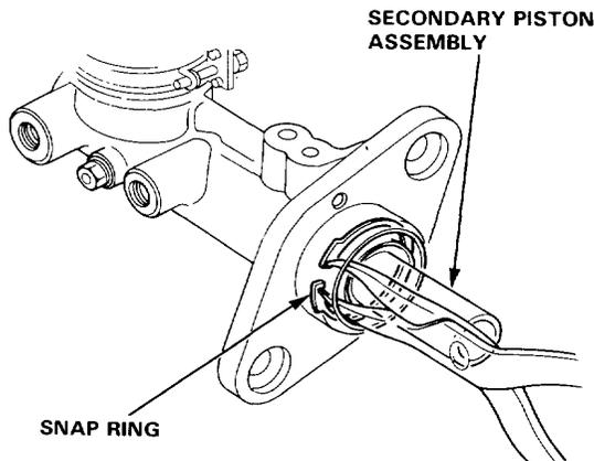
3. Remove the stop bolt while pushing in the secondary piston assembly.
