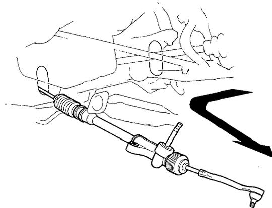
13. Slide the gear box right so that the left tie rod clears the bottom of the rear beam, then remove the gearbox.
