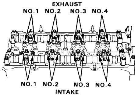
2. Set the No. 1 piston at TDC. "UP" marks in the pulleys should be at top, and the TDC grooves on back side of pulley should align with cylinder head surface. The distributor rotor must be pointing towards No. 1 plug wire.
