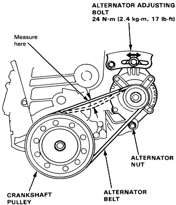
2. Loosen the alternator adjusting bolt and nut.
