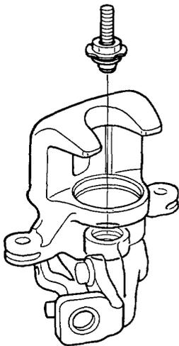
12. Install the brake spring compressor (special tool) as shown.
