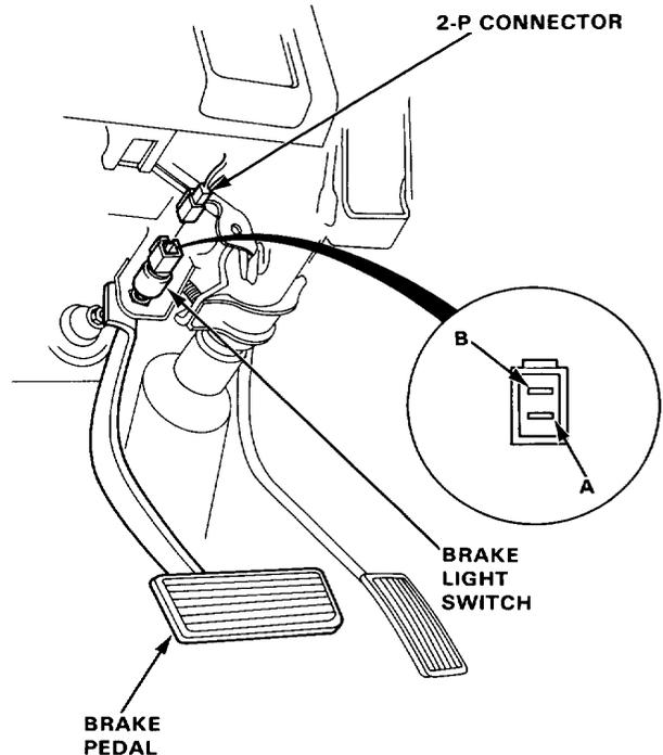
3. Check for continuity between the A and B terminals. There should be continuity with the brake pedal pushed.
