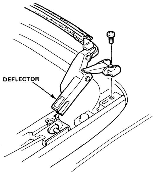
2. Install the deflector in the reverse order of removal. Adjust the deflector.
