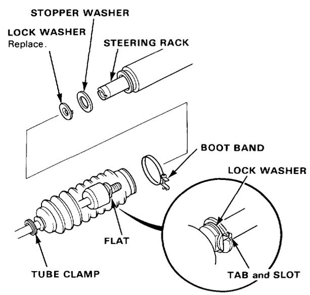
13. Install the boots and secure with boot band and tube clamp.
