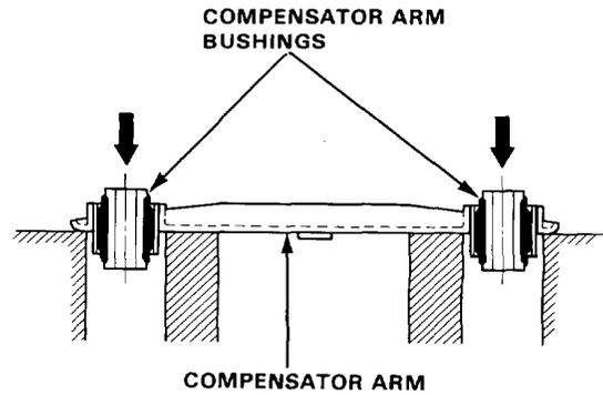
2. Drive in the compensator arm bushings from the direction indicated.
