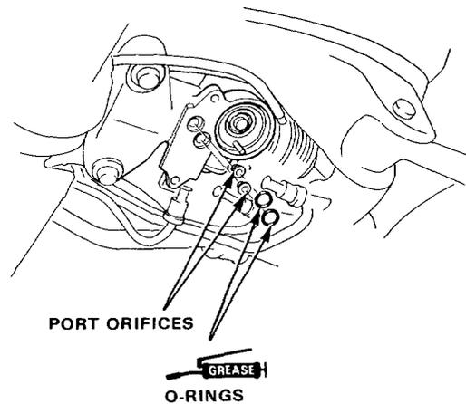
7. Install the O-ring to the valve body unit, then install the valve body unit on the gear housing with the two 6 mm bolt.
