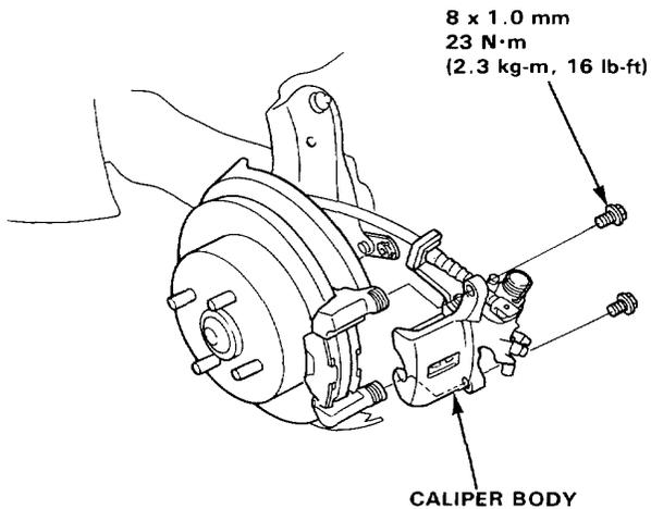
4. Remove the pads and measure the thickness of each brake pad lining using a vernier caliper.
