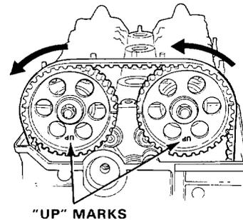
8. Rotate crankshaft 180° counterclockwise to bring No. 2 piston to TDC. "UP" marks should be at intake side. Distributor rotor should point to No.2 plug wire. Adjust valves on No.2 cylinder.
