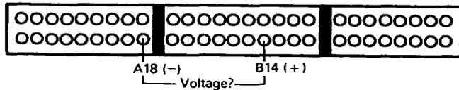
Does the voltage decrease when headlight and rear defogger are turned on ?
