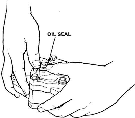
15. Install the new oil seal in the pump front cover; get it started by hand, then use a 19 mm socket to push it in the rest of the way.
