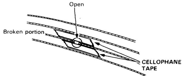
3. Using a small brush, apply heavy coat of silver conductive paint extending about 1/8 in. on both sides of the break. Allow 30 minutes to dry.
