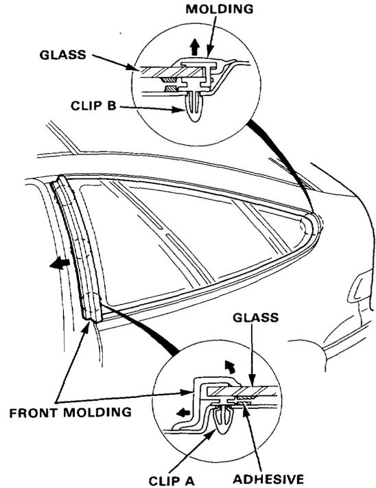
4. Remove the quarter glass molding if the glass is to be reused.
