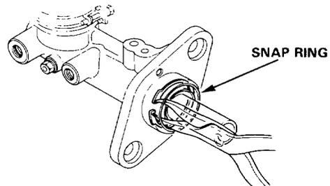
5. Install a new rod seal.
