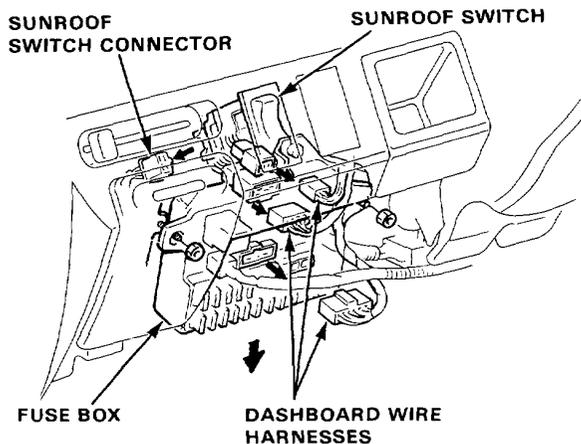
NOTE: Remove the fuse box mounting nuts, then lower the fuse box, if necessary.
