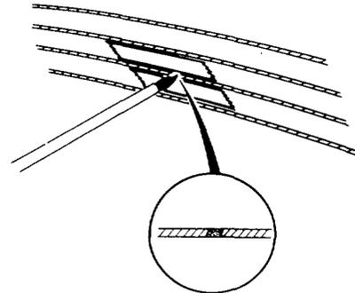
4. Check for proper operation with a voltmeter (approximately 6 V at the mid-point).
