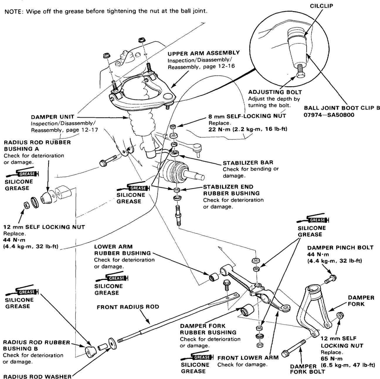
CAUTION: Do not interchange the radius rod rubber bushings. The thick bushing should be installed in front position.
