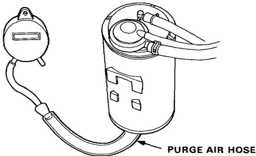
6. Raise engine speed to 3,500 min<sup>-1</sup> (rpm). Vacuum should appear on gauge within 1 minute.
