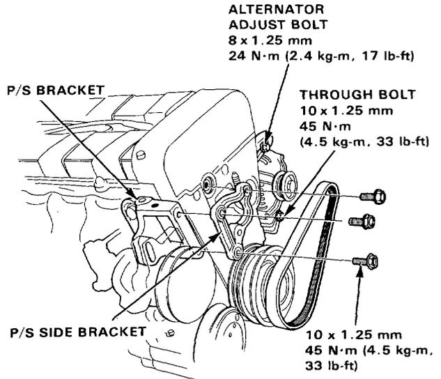
6. After installation, adjust the tension of each belt. See page 5-6 for alternator belt tension adjustment. See page 5-7 for A/C compressor belt tension adjustment. See page 5-7 for P/S pump belt tension adjustment.
