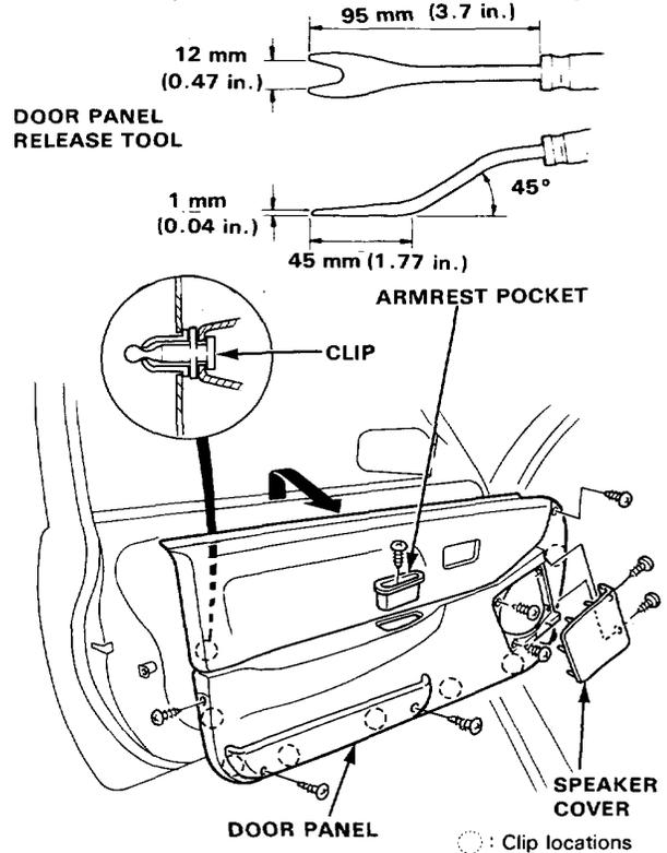
5. Remove the screws, then remove the speaker and door panel bracket.
