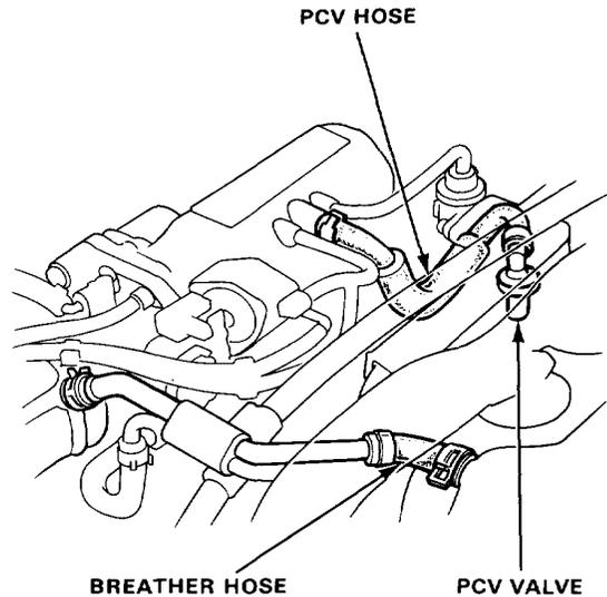
2. At idling, make sure there is a clicking sound from the PCV valve when the hose between PCV valve and intake manifold is lightly pinched with your fingers or pliers.
