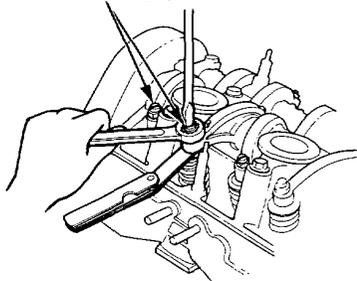
5. Tighten locknut and check clearance again. Repeat adjustment if necessary.
