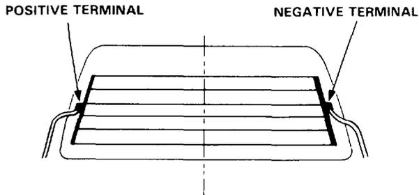
2. Check for continuity between the negative terminal and body ground.
