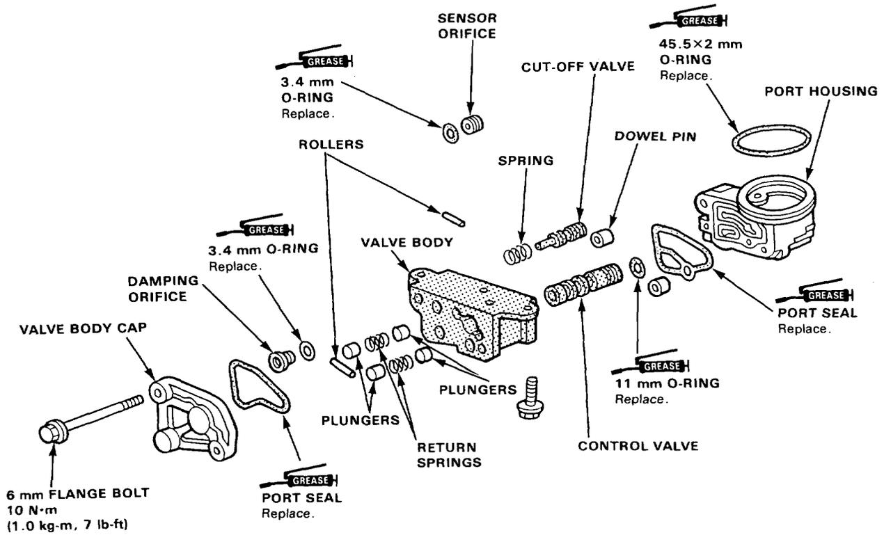
NOTE: If the Valve Body is damaged, it must be replaced as a set, with the Cut-off Valve and Control Valve (shaded parts).
