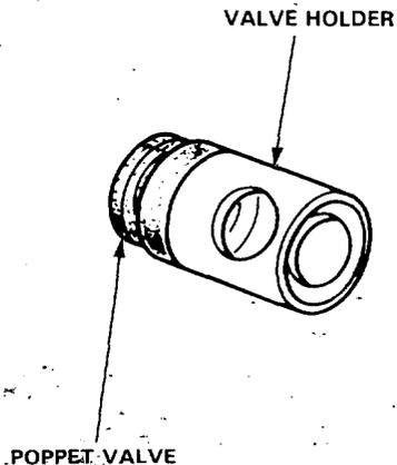
2. Install the valve holder, inner valve spring, outer valve spring and spring seat on the push rod.
