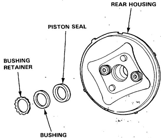
NOTE: Make sure the lip of the seal is facing in, as shown in drawing below.
