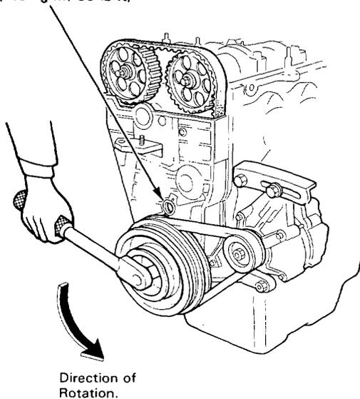
3. Rotate crankshaft counterclockwise 3-teeth on camshaft pulley to create tension on timing belt.
