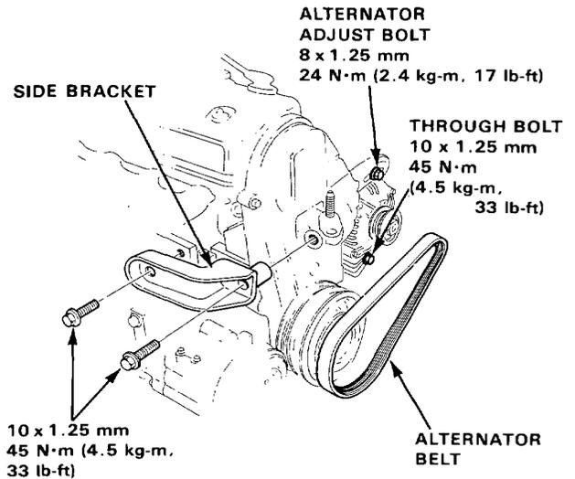
5. After installation, adjust the tension of each belt. See page 5-6 for alternator belt tension adjustment. See page 5-7 for A/C compressor belt tension adjustment.
