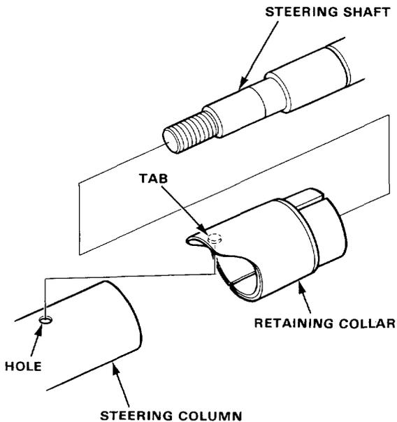
3. Insert the steering shaft into the steering column from the bottom.
