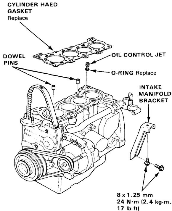
3. Install the intake manifold and tighten the nuts in a criss-cross pattern, beginning with the inner nuts.
