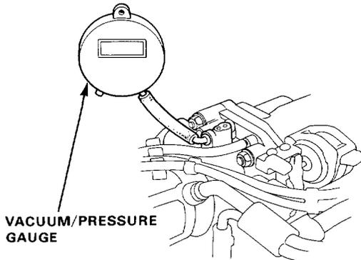
3. Allow the engine to idle and check that the gauge indicates no vacuum.
