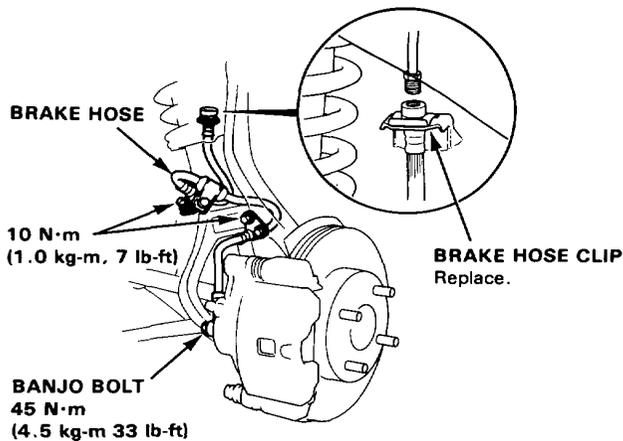
5. Install a new brake hose clip to the brake hose.
