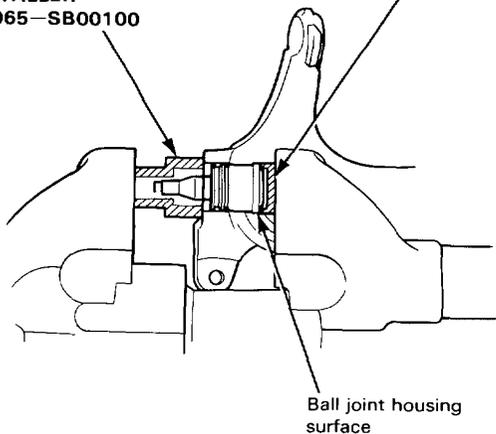
8. Install the 40 mm circlip.
