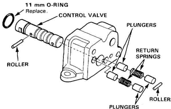
15. Remove the plungers, return springs and control valve from the valve body.
