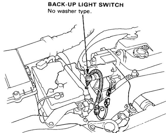
3. Install the back-up light switch.
