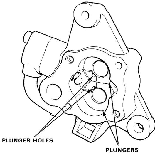
2. Coat the inside of the plungers with power steering fluid.
