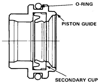
2. Install the piston assemblies in the master cylinder.
