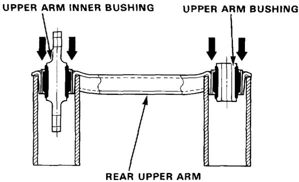
2. Mark a scribe line on the upper arm inner bushing so that it is in line with the bolt mounting surface.
