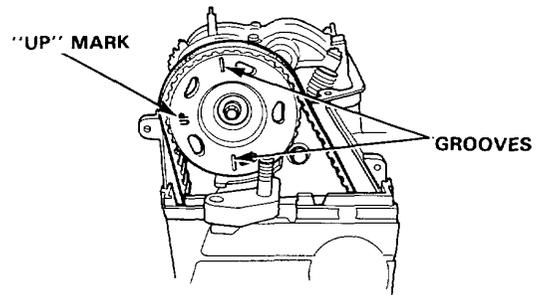
7. Rotate crankshaft 180° counterclockwise to bring No. 4 piston to TDC. Both TDC grooves are once again visible and distributor rotor points to No.4 plug wire. Adjust valves on No.4 cylinder.
