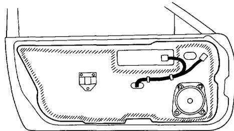
5. Install the regulator handle so it points backward, and up at a 45 degree angle with the window closed.
