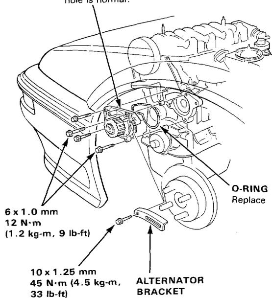
3. Install the water pump in the reverse order of removal.
