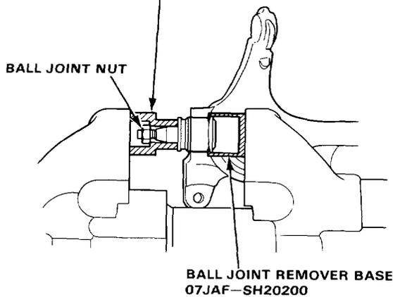
6. Place the ball joint in position by hand.
