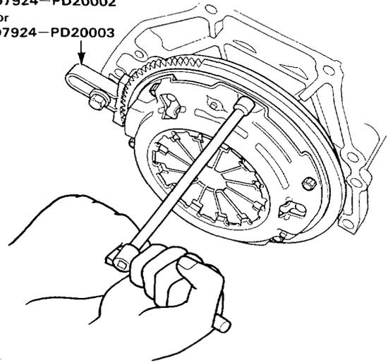
5. Inspect the pressure plate surface for wear, cracks, or burning.
