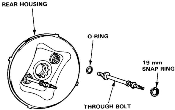
12. Install the booster piston on the rear housing aligning their tabs and slots.
