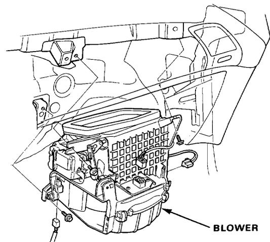
6. Install the blower in the reverse order of removal and make sure there is no air leakage.
