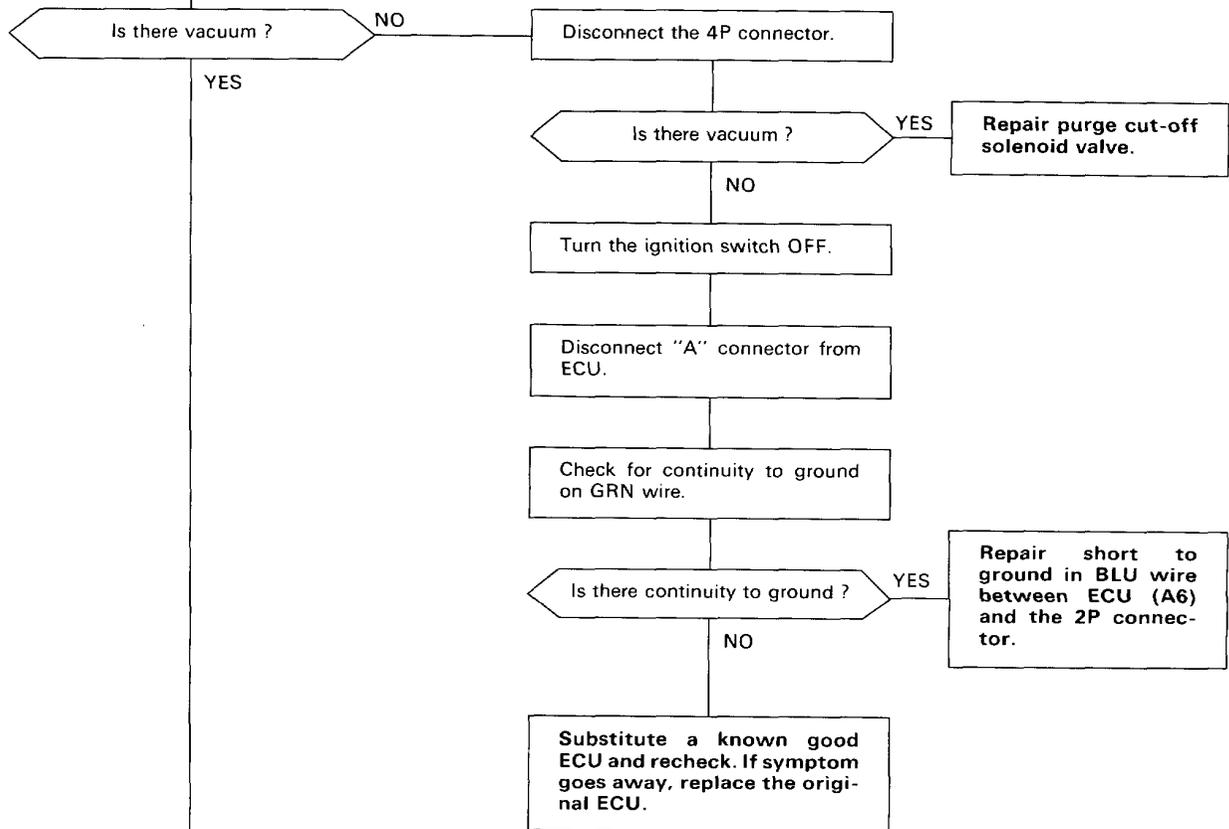
Connect a vacuum gauge to canister purge air hose.
