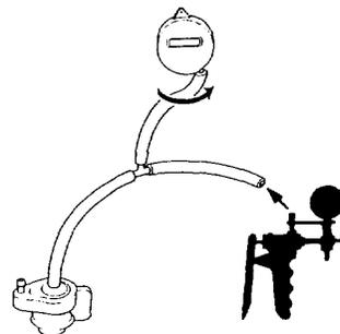
5. Slowly pressurize the vapor line while watching the gauge. Pressure should stabilize at 10 to 25 mmHg (0.4 to 1.0 in. Hg).
