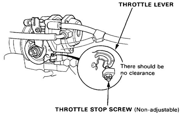
Replace the throttle body if there is excessive play in the throttle valve shaft or if the shaft is binding or sticking.
