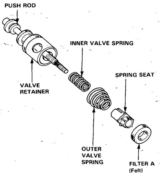
3. Install a new filter A (felt) on the push rod and secure with a new E-clip.
