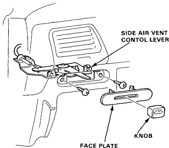
7. Remove the 3 screws attaching the function panel to the dashboard.
