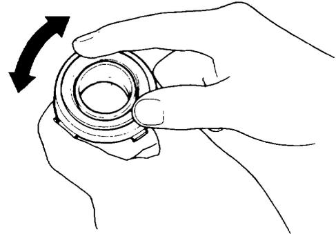
5. Replace the bearing with a new one if there is excessive play.
