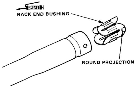
3. Apply grease to the steering rack.
