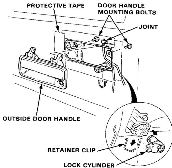
11. Pull the outside door handle out, and pry the joint off the handle with a flat-tip screwdriver. Remove the handle from the rod.
