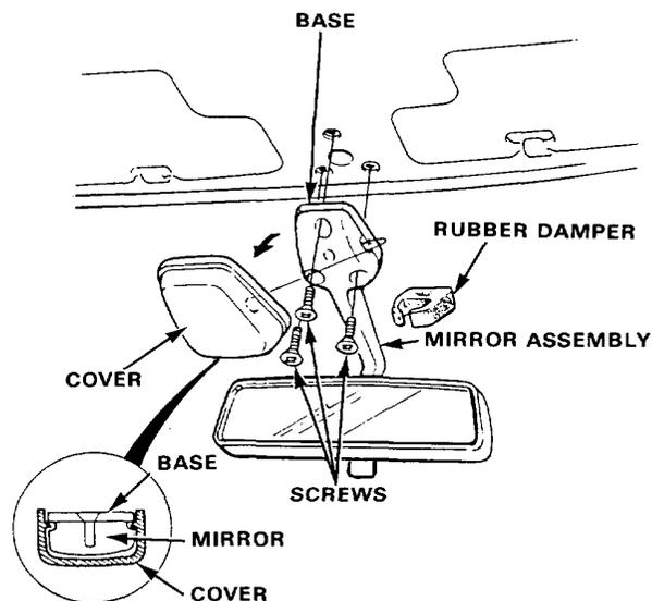
3. Remove the 3 mounting screws from the mirror base, then remove the mirror assembly.
