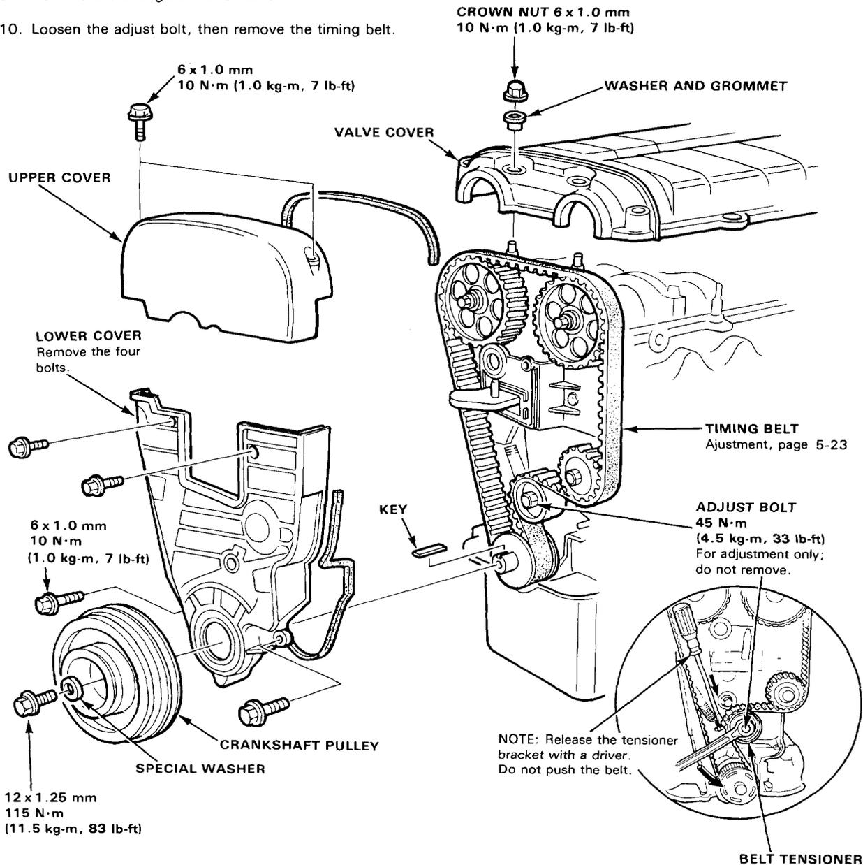
11. Install in the reverse order of removal; adjust the valve timing (page 5-26).
