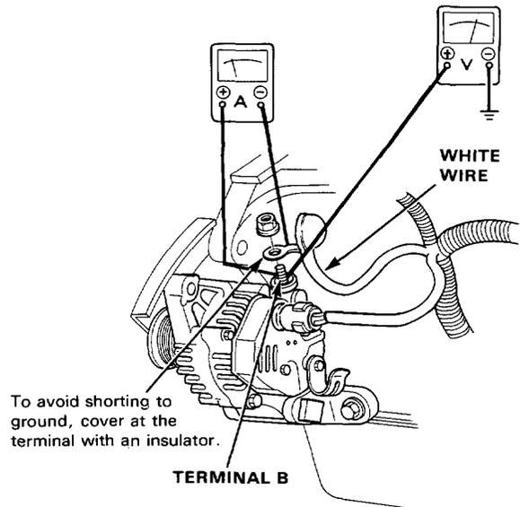
4. Start the engine, and turn on the headlights, blower motor, rear window defogger, etc.
