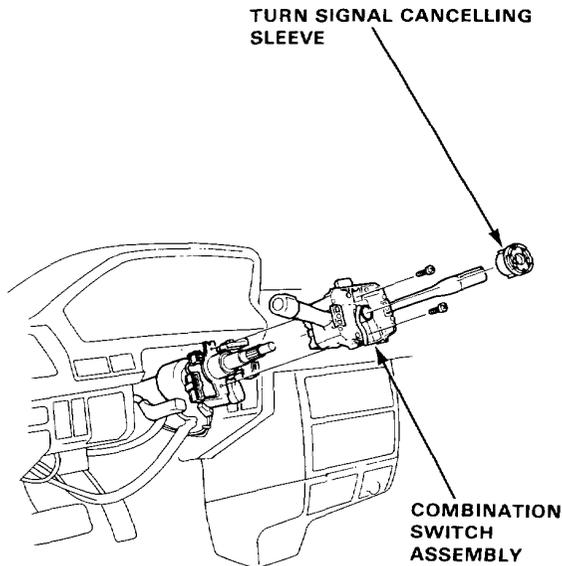
10. Remove the lower column bracket.
