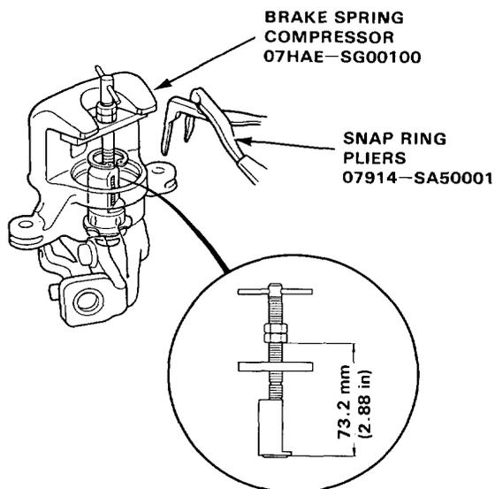
11. Remove the brake spring compressor from caliper body.
