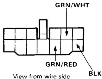
Connect the GRN/WHT and GRN/RED terminals to BLK terminal using a jumper wire. Turn the ignition switch ON.
