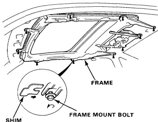
2. Side-to-side fit of sunroof seal can be adjusted by moving it right or left by hand.
