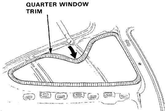
2. From inside the car, use a knife to cut through the glass adhesive all the way around.
