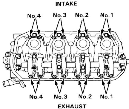
2. Set No. 1 piston at TDC. "UP" mark on the pulley should be at top, and TDC grooves on the pulley should align with cylinder head surface. The distributor rotor must be pointing towards No. 1 plug wire.
