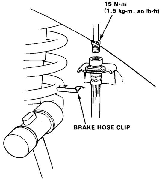
7. Connect the brake hose to the caliper.
