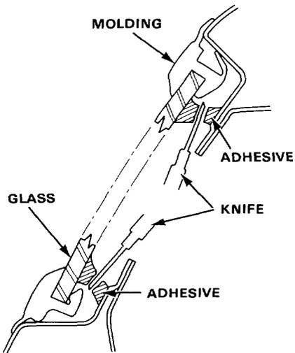
3. As an assembly, pry the glass and upper and front moldings away from the car at the clip points shown.
