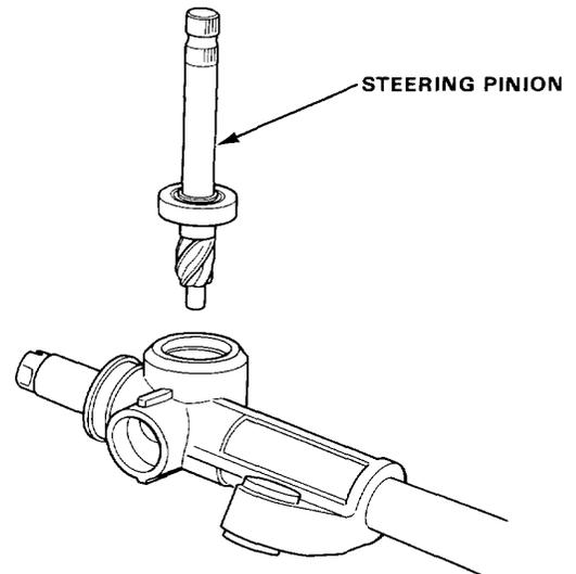
6. Install the 35 mm snap ring securely in the gear housing groove.
