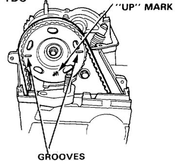
8. Rotate crankshaft 180° counterclockwise to bring No. 2 piston to TDC. The "UP" mark should be at intake side. Distributor rotor should point to No. 2 plug wire. Adjust valves on No. 2 cylinder.
