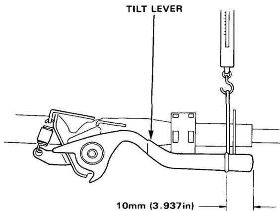
10. If the force measured is not within the specification, remove the tilt lock plate then reset it in the position where the correct force can be obtained.
