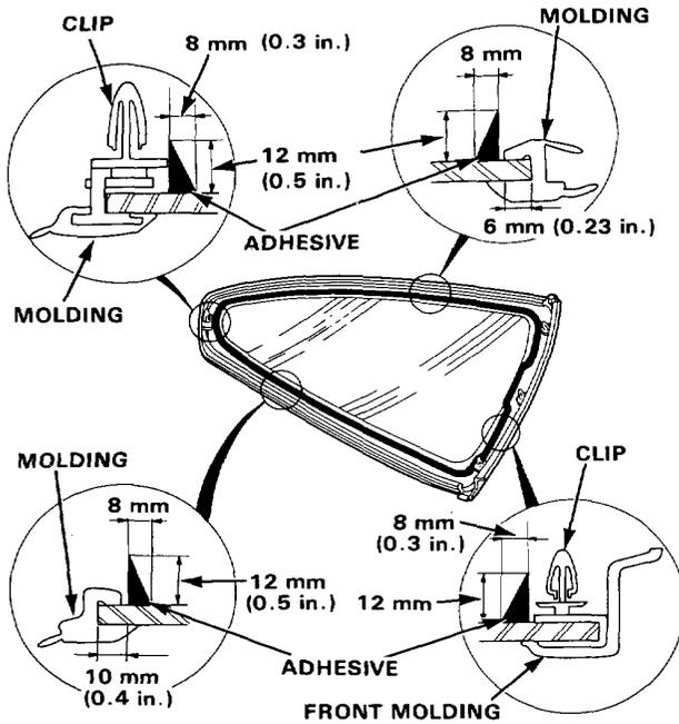
12. Use suction cups to hold the glass, then set it on the adhesive. Lightly push on the glass until its edges are fully seated on the adhesive all the way around.
