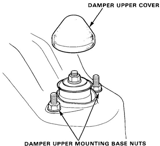
4. Remove the damper mounting bolt.
