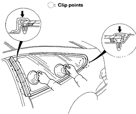
13. Scrape or wipe the excess adhesive off with a putty knife or gauze.
