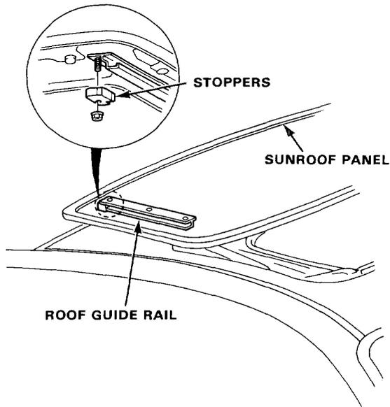
3. Remove the front mounting bolts. Remove the sunroof panel from the rear slide bracket by sliding it forward by hand.
