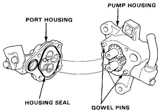
6. Remove the dowel pins from the pump housing and remove the housing seal and O-ring from the port housing.
