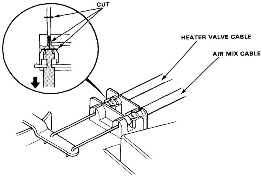
NOTE After assembly check that the air mix lever slides smoothly.
