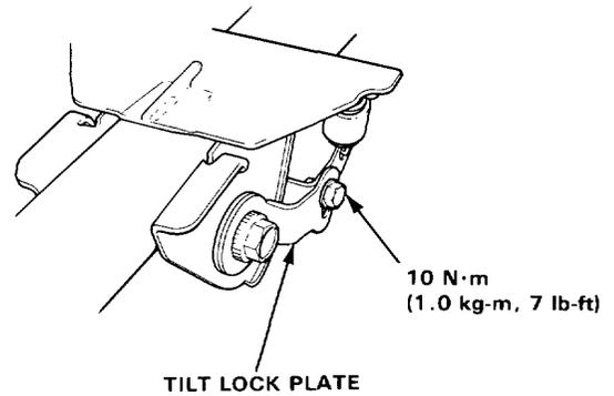
11. Tighten the tilt adjusting bolt.
