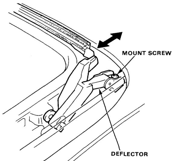
3. Adjust the deflector forward or backward so the edge of its blade touches the front edge of the roof opening evenly.
