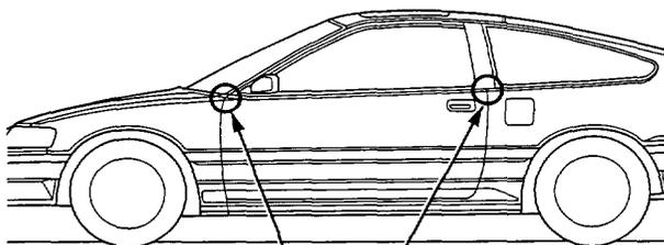
The door and body edges should be parallel.
