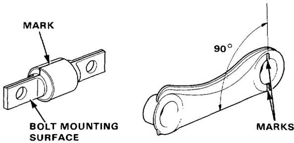
4. Drive in the upper arm inner bushing with the marks aligned.
