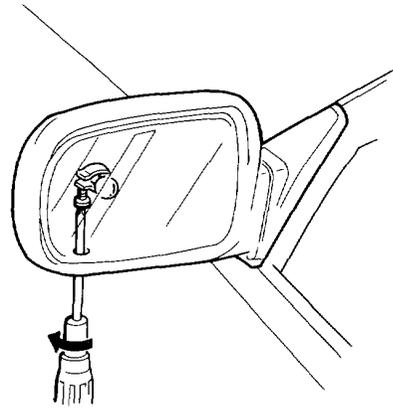
2. Carefully pry out the mirror with a flat-tip screwdriver as shown.
