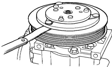
NOTE: The shims are available in two sizes: 0.2 mm and 0.5 mm of thickness.
