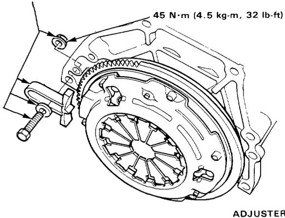
When installing the ring gear holder,
