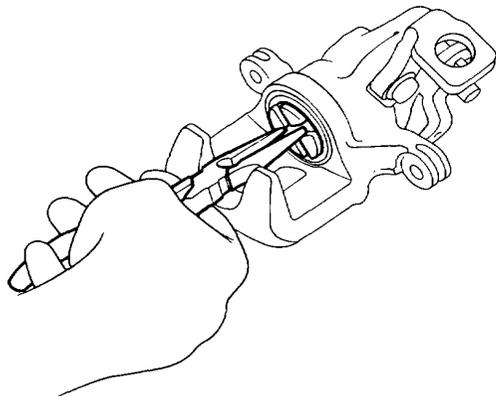
7. Remove the circlip, then washer, adjusting spring A, and the adjusting nut from the piston.
