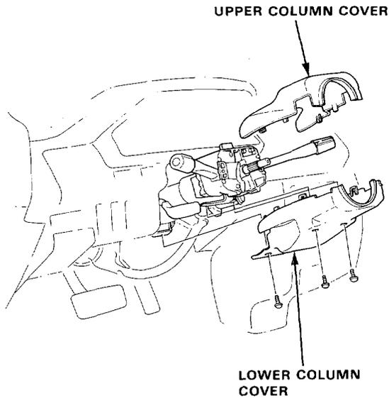
8. Disconnect each wire coupler from the combination switch.
