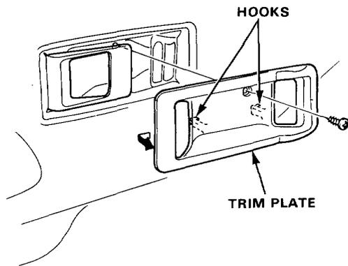
2. Remove the power window switch, if equipped, from the trim plate by removing the 4 screws.
