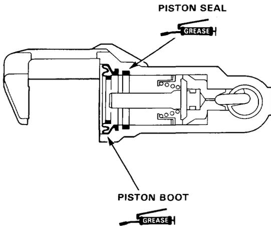
18. Coat the outside of the piston with silicone grease, and install it on the adjusting bolt while rotating it clockwise.
