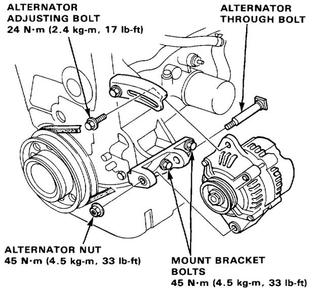
6. If necessary, remove the mount bracket bolts, and the upper and lower mount brackets.
