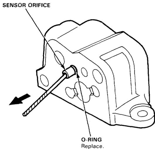
20. Using 1.5 mm (1/16") drill bit, push the damping orifice and O-ring out of the valve body.
