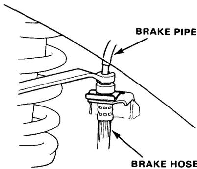
3. Remove and discard the brake hose clip from the brake hose.
