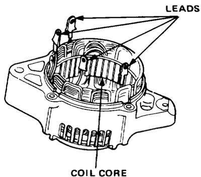
3. If the coil fails either continuity check, replace the stator.
