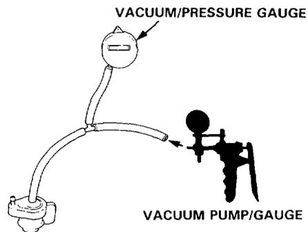
3. Slowly draw a vacuum while watching the gauge. Vacuum should stabilize at 15 to 30 mmHg (0.6 to 1.2 in. Hg).
