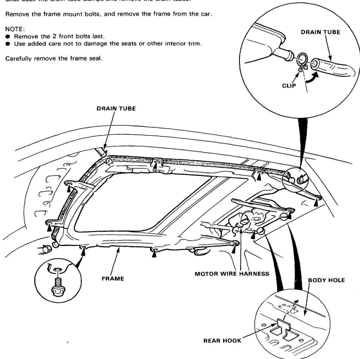
6. To install, insert the frame's rear hooks into the body holes, then install parts in the reverse order of removal.
