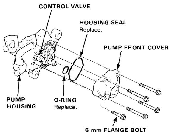
3. Remove the housing seal from the pump housing.
