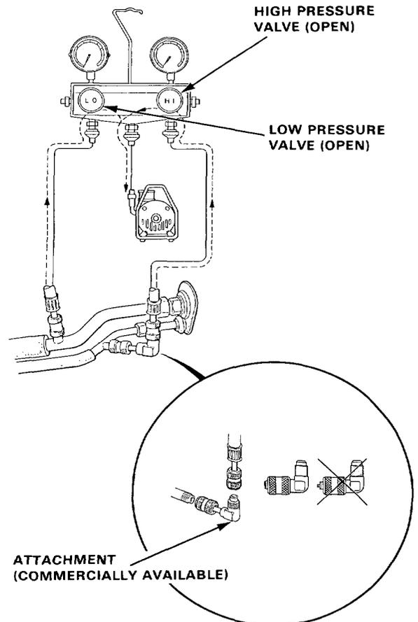
NOTE: Set the attachment to the gauge hose at high pressure side, then install the gauge set as shown.
