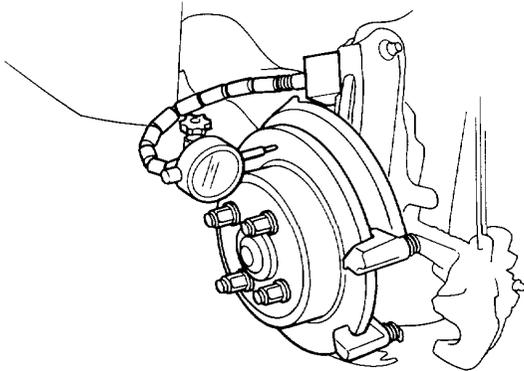
9. Using a micrometer, measure the rear brake disc thickness at eight points, approximately 45 apart and 10 mm (0.39 in) from the outer edge of the disc.
