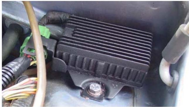
2. When you get the Injector Resistor Box, be sure to get the connector that plugs into it (the green connector in the picture), just in case your ZC harness has the connector cut off. This connector will have five (5) wires coming out of it – one yellow with a black stripe and four (4) red with a black stripe. Get as much length of these wires as you can.
