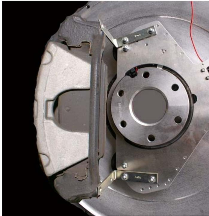
Here is a photo of one angle bracket mounted in position. Note the cable tie securing the bracket against the caliper body.
