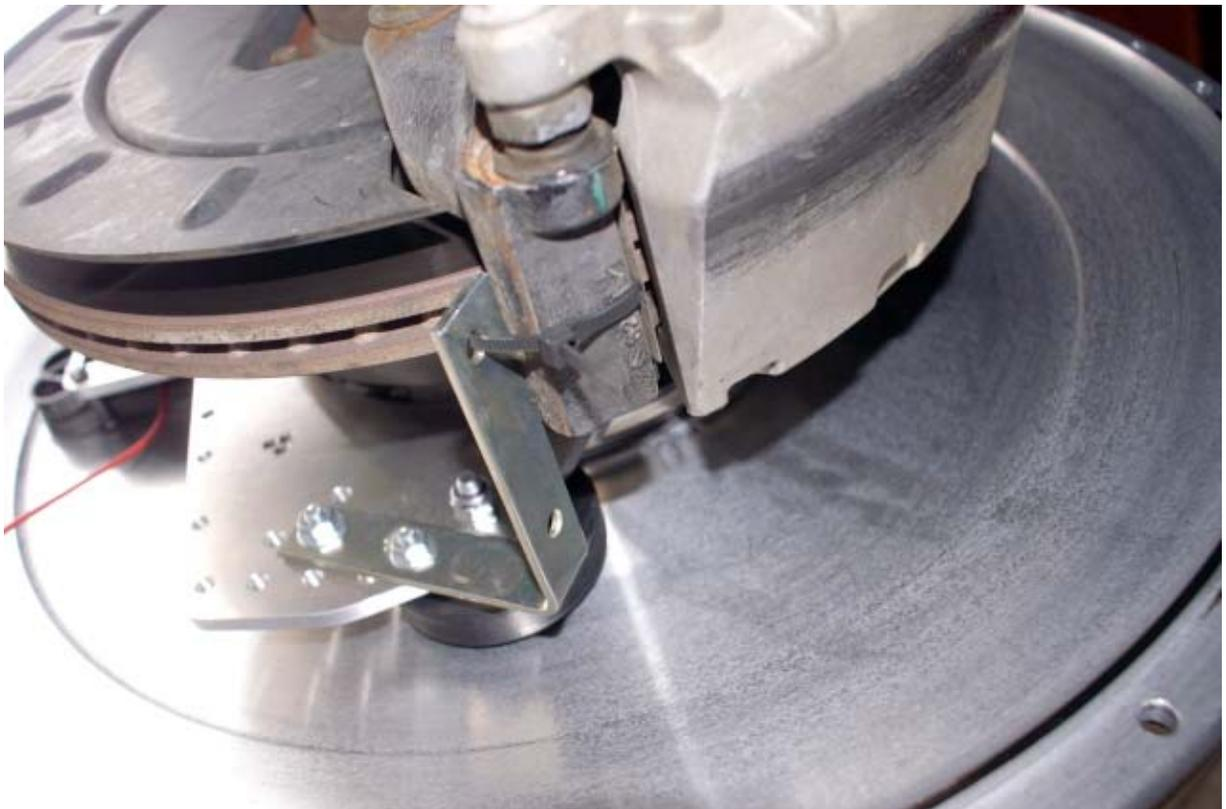
You may find it useful to use standard angle brackets, or you may bend your own brackets using flat bar stock, or heavy duty perforated flat stock. Note that you may have to drill additional holes in the trolley plate to secure the angle bracket.
