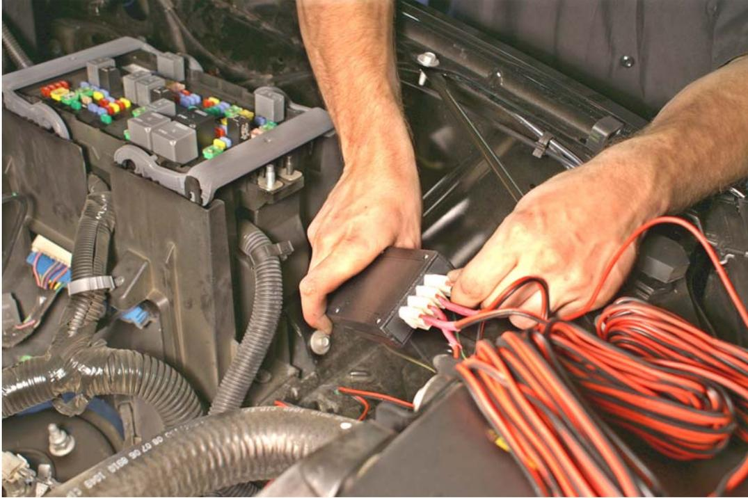
The black wire is the ground and it must be attached to a solid ground point as close to each wheel's hub or spindle as practicable. Generally, it is possible to find some non-critical fastener (such as a mounting bracket bolt) which may be loosened to accommodate the ground wire termination. Never loosen, remove, or attach to any hardware relating to the vehicle's brake system or suspension.
