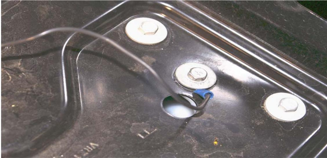
Plug the heavy power cable into the power block. You will notice that there is a black ground wire which is attached to this cable. There is also a short black ground wire which is attached to the power block. Both of these wires will need to be connected to a chassis ground. Identify a suitable ground point and secure the two ground wires to chassis ground.
