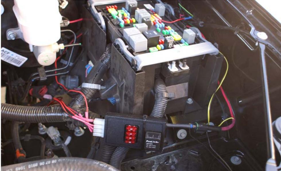
Test the system to make sure the wiring has been completed correctly. To test, turn the vehicle's ignition to 'on' (make sure you do not start the engine), flip the rocker switch to the 'on' position (it should illuminate) and use a test light or multi-meter to verify that +12VDC is present at each wheel's red wire (spade connector) and the black wires are properly grounded. Flip the switch to 'off' and turn off the vehicle ignition.
